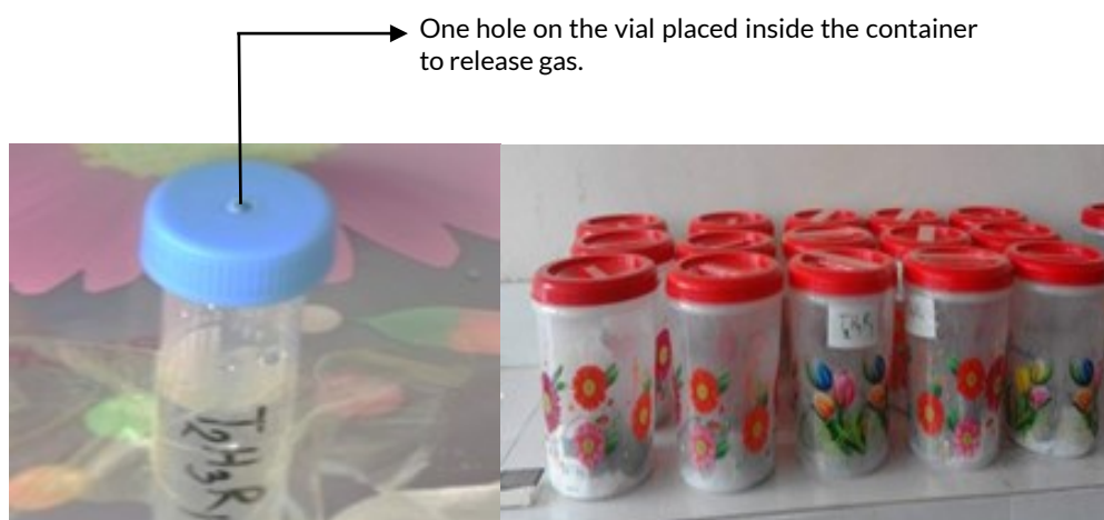
Figure 1. One vial placed inside the container (left side and container set up for the experiment shown (right side))
