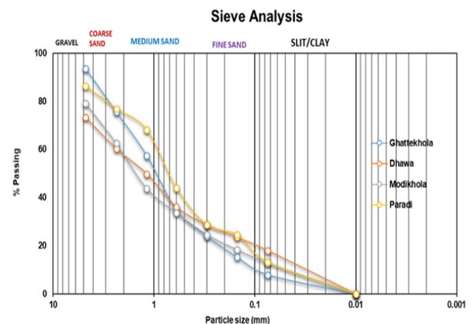
**Figure 4.** Grain size distribution analysis of soil samples.
